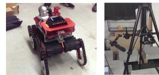
The Quince robot, left, is also being used at the University of Tokyo for research on autonomy and computer vision. Acoustic analysis of materials is represented on right.
