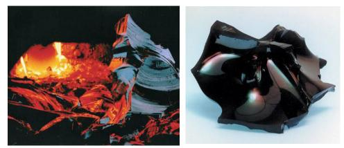
Examples of waste after the vitrification process is completed by the WTP.
