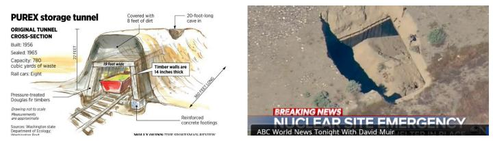
A diagram of a cross-section of the smaller PUREX tunnel (left), showing its construction. An overhead picture (right)
