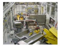
A work cell containing robot arms and conveyors is used to sort mixed waste.
