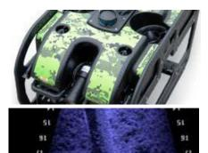
Example ROV and high-resolution SONAR images of an underwater pipe.
