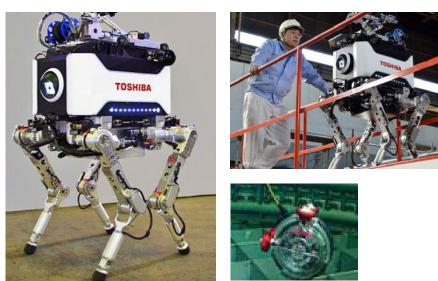
Toshiba quadruped robot that can climb stairs and carries a remote, tethered robot for inspection. An underwater inspection robot, far right, inspects inside the reactor vessel.
