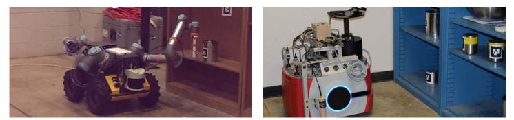
A bi-manual mobile robot for inspecting radiological samples in a warehouse environment, left. Another warehouse inspecting robot "sniffs" the floor to look for possible spills and other forms of localized contamination, right. This robot tirelessly searches the entire floor and maps evidence of contamination for future comparisons.
