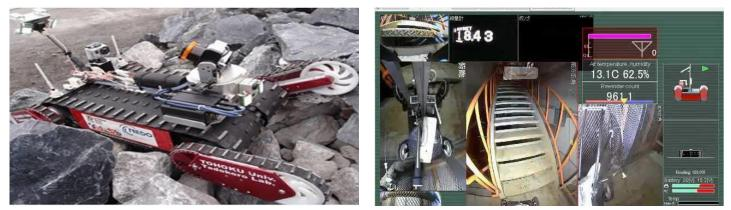
Quince robot on a rubble pile (left) and in-use at Fukushima Daiichi (right).
