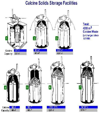
Schematics for seven concrete silos show the varied tank configurations, pipe networks, and calcine capacities of each silo.
