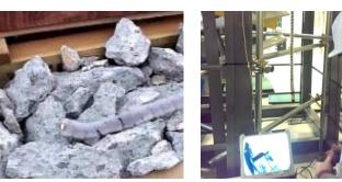
Tohoku's Active Scope Camera (ASC) on a pile of rocks in the lab (left) and the operator console with PlayStation controller (right).
