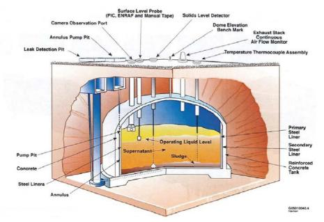
Cut-away of a typical double-shell tank.
