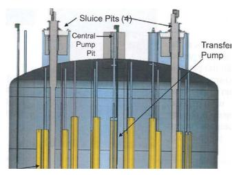
Example of a tank with additional internal obstacles such as piping for cooling, etc.
