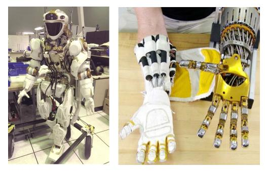
Valkyrie is the latest NASA/JSC humanoid that competed in the DARPA Robotics Challenge. Right, the RoboGlove, a "power glove" for human augmentation to reduce fatigue, is derived from Valkyrie. (right image courtesy NASA)
