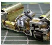
Figure 4.20: An example of the shape-shifting, tread-driven robot that was deployed into the PCV in April of 2015.
