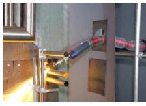
The LaserSnake cutting a pipe in a mock cell.
