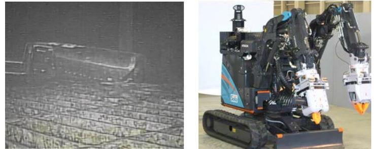
Figure 4.21: Actual image of the first deployed robot inside the PCV from the perspective of the second deployed robot. The first robot died after about three hours.
