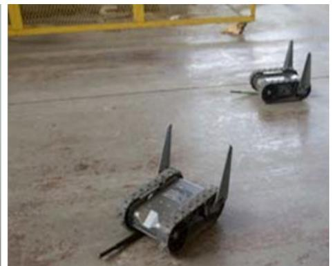
Endeavor showcased a product demonstration of three of their 110 FirstLook robots. The 110 FirstLook is an expandable, lightweight robot that can provide immediate situational awareness, perform persistent observation, and investigate dangerous and hazardous material while the operator is in a remote, safe setting. The platform is robust, which was demonstrated by having members of the audience throw the vehicle as far and as hard as possible, without damaging it.
