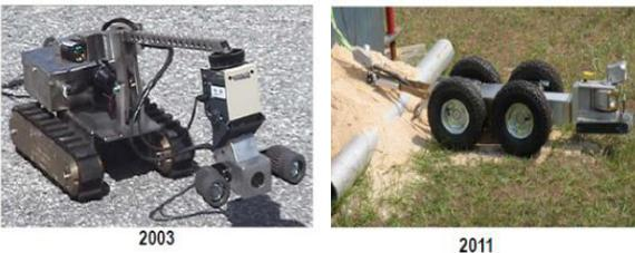
Two of five different robots developed for the H-Canyon Exhaust Tunnel at Savannah River. (reprinted from Reid 2015)
