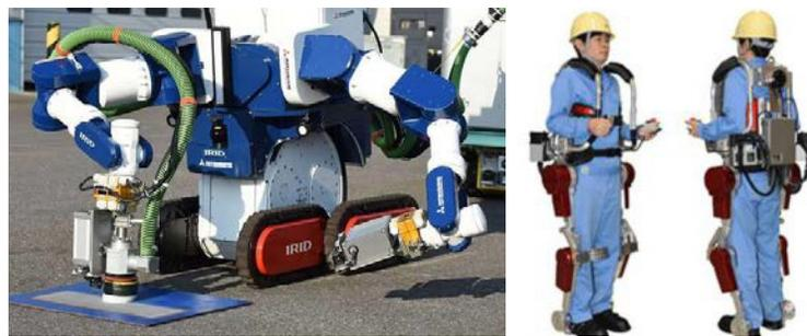
Mitsubishi MEISTER two-armed robot with heavy duty versions of the PA-10 commercial manipulator (left). The MHI power suit allows heavy loads to be borne by the exoskeleton (right).
